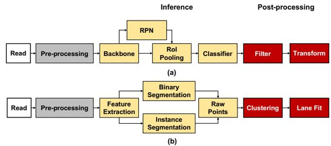
Fig. 3. Generalized two-stage object detection (a) and lane detection (b).
