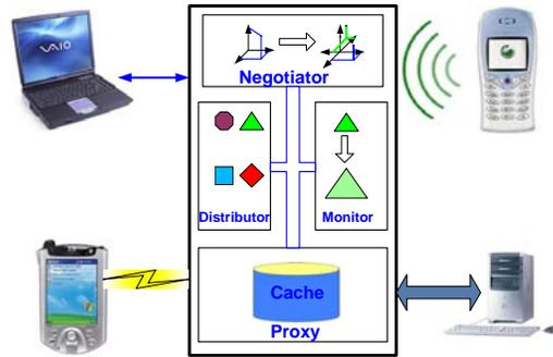
Fig. 2. The structure of gateway.
