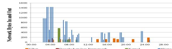
Fig. 15: Network bytes in and out of Android using 3G during test 2
