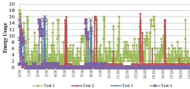
Fig. 3: Energy usage of iPhone using Wi-Fi
