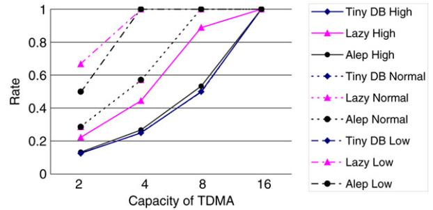
Fig. 7. Comparison of the successful delivery rate vs. TDMA capacity, the number of maximum delivered messages in one TDMA round.
