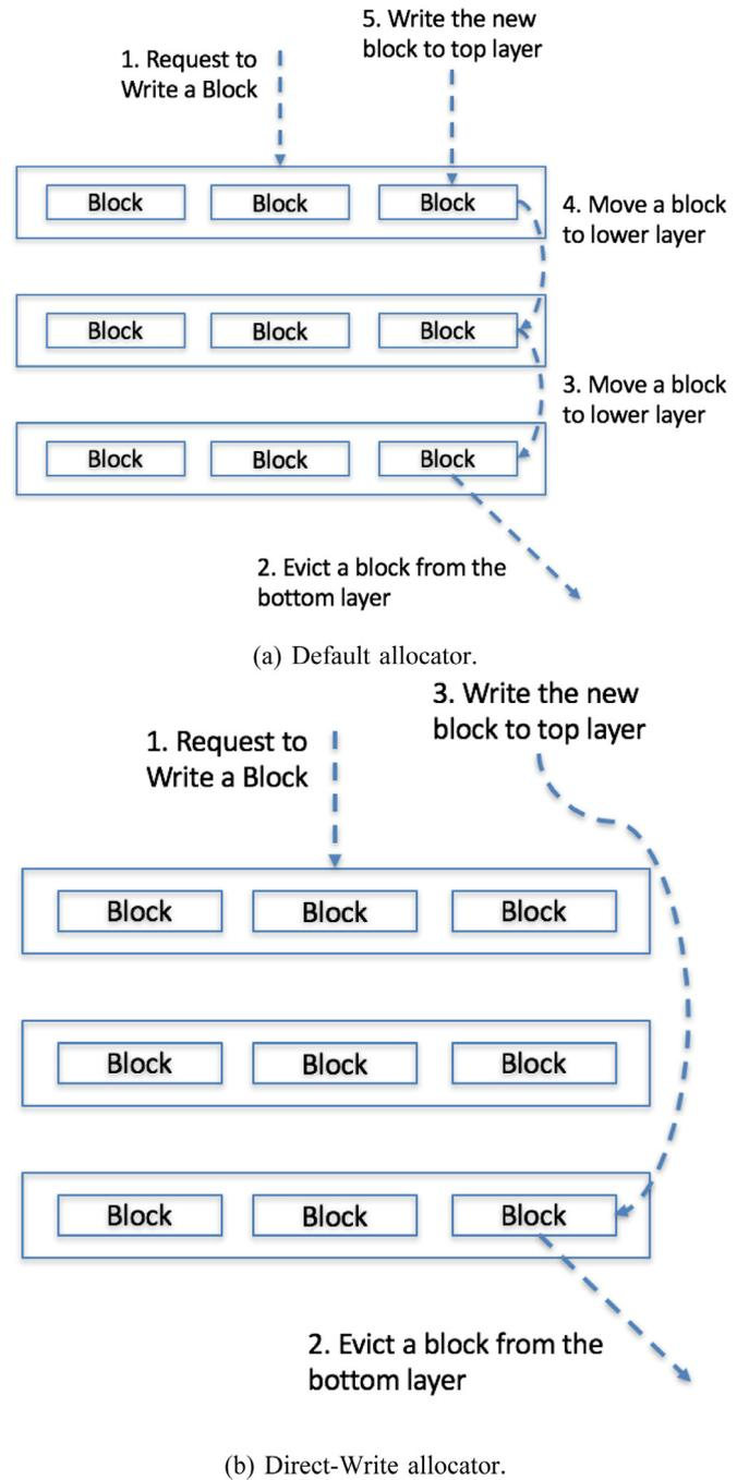
Fig. 11. Write optimization in  $\pi$ -Hub.
