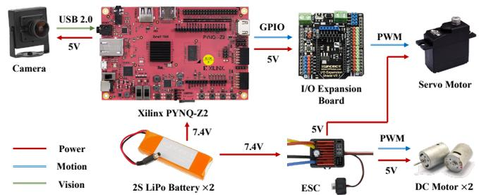
Fig. 3. HydraMini Hardware Design.
