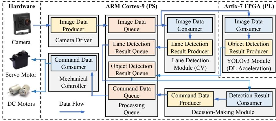
Fig. 8. Autonomous Driving using Traditional Methods.
