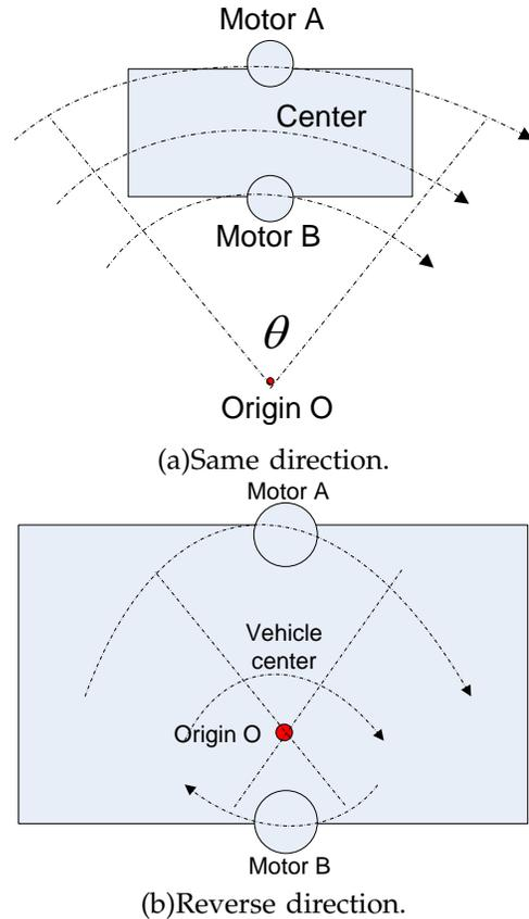
Fig. 4. Travel distance with different-pace motors.
