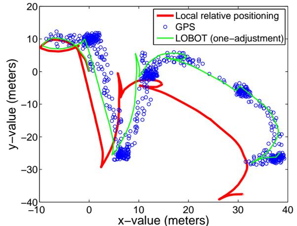
Fig. 12. Outdoor experiments with one-time GPS-augmentation.
