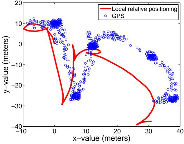
Fig. 5. Drift in local relative positioning.
