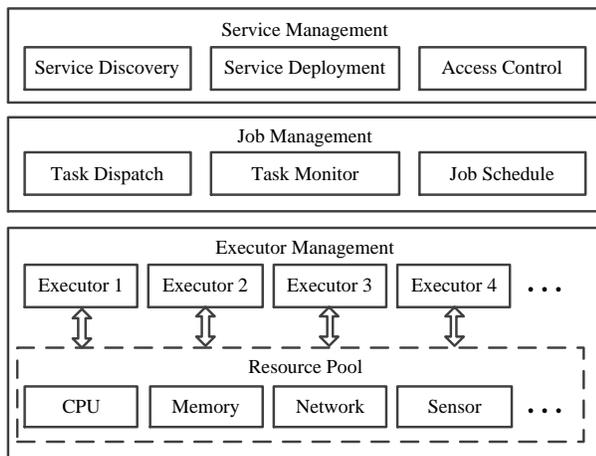
Fig. 4. *Firework's* new architecture, including its extensions.
