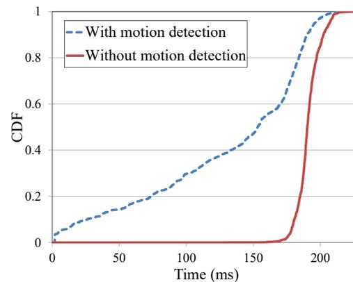
Fig. 2. The time cumulative distributive function (CDF) of license plate detection and recognition on an Amazon EC2 t2 node.
