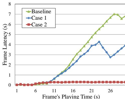
Fig. 13. Frame latency over time under the collaboration of local edge nodes.
