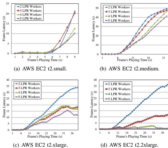
Fig. 10. Frame latency over time in different types of AWS nodes with different numbers of LPR workers.
