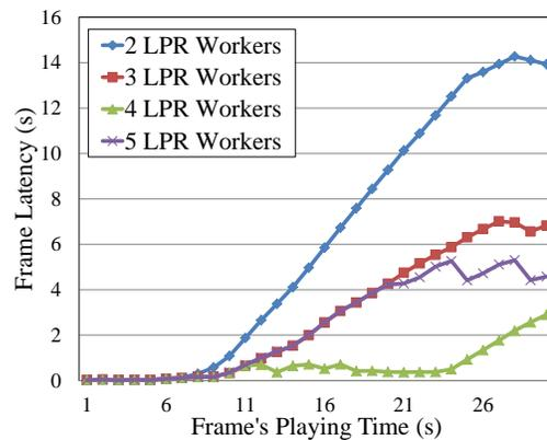
Fig. 11. Frame latency over time on a Dell OptiPlex with different numbers of LPR workers.
