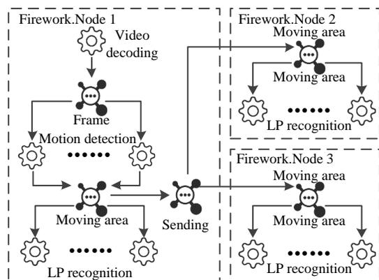
Fig. 6. An example for using message queues in the *Firework* prototype.
