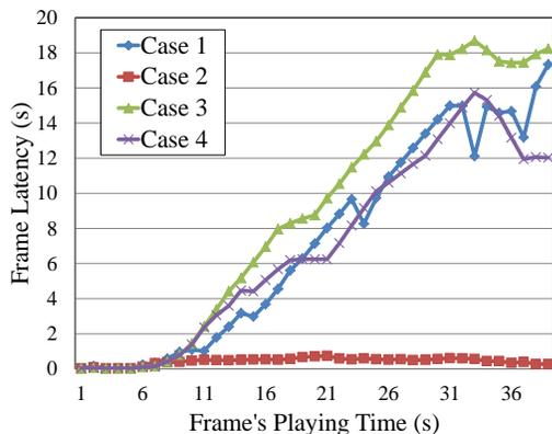
Fig. 12. Frame latency over time as AWS nodes collaborate.
