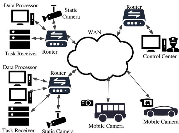
Fig. 7. The network settings of an A3 application scenario.
