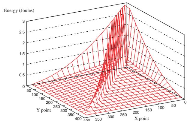
(b) Energy consumption of sensors using IQ
