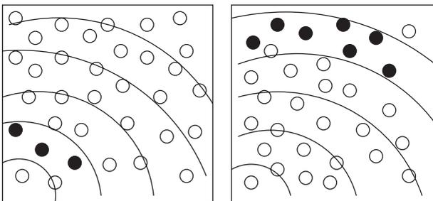
(a) The sensors near the sink are dead (b) the sensors far from the sink are dead
