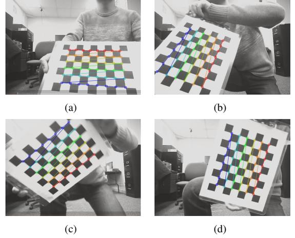
Fig. 7: Checkerboard on camera view in different orientation.
