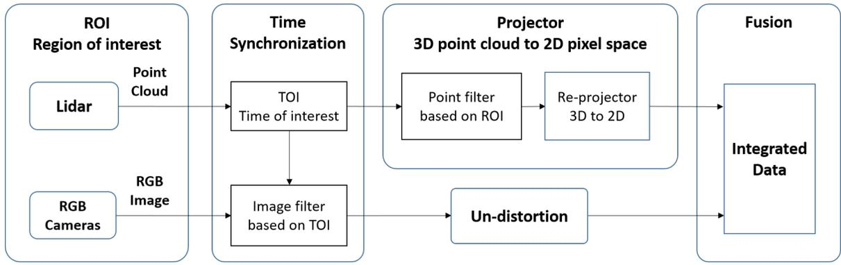
Fig. 2: FlowChart of the data synchronization in HydraView.
