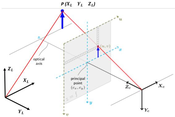
Fig. 3: Pinhole camera model.
