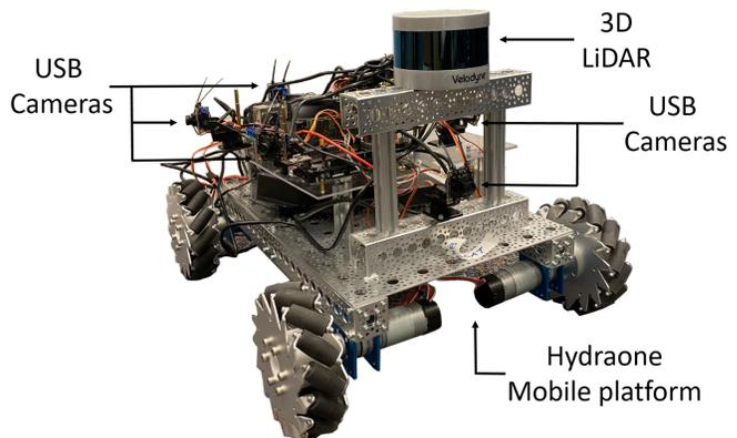
Fig. 1: Overview of HydraView with HydraOne Mobile platform.
