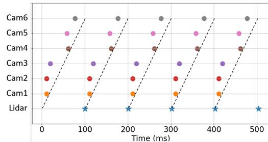
Fig. 14: Synchronized six cameras data and LiDAR data.
