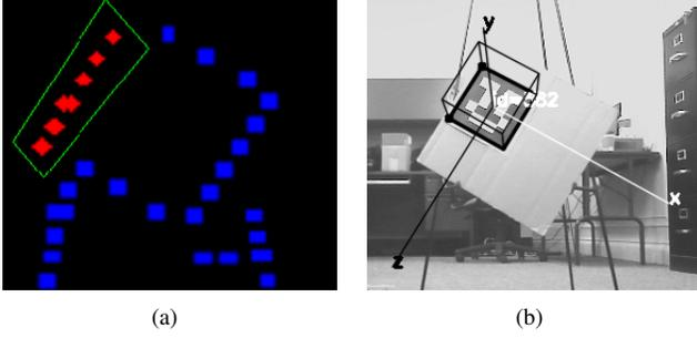
Fig. 6: (a) 3D points represent the edge of marker captured by LiDAR; (b) The position of ArUco marker captured by camera
