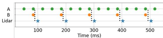
Fig. 12: Synchronization for one camera.
