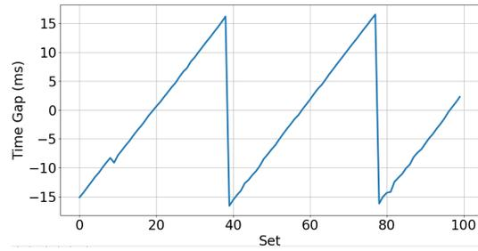
Fig. 13: Time gap between synchronized image and corresponding LiDAR data.
