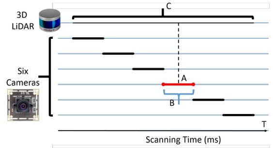
Fig. 4: Corresponding time period for each camera in one scanning cycle.
