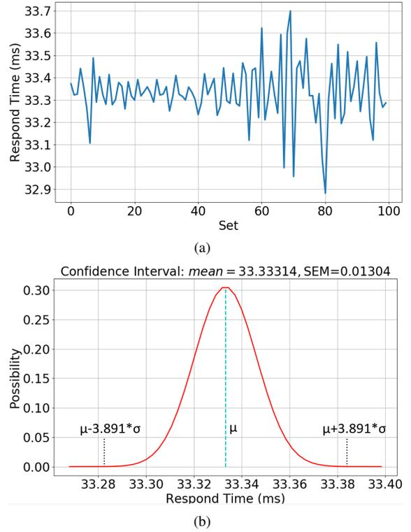
Fig. 5: (a) Distribution of responding time of camera; (b) Confidence intervals of responding time of camera
